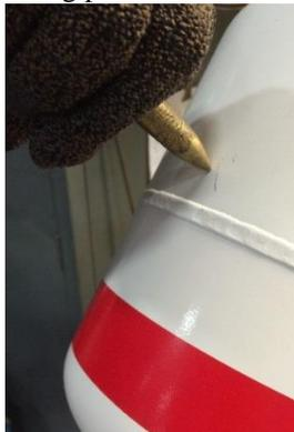
**Figure 4. Placement of Non-sparking Pick for Piercing**
