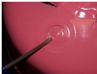
**Figure 1. Placement of Screwdriver for Piercing**
