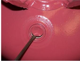
**Figure 2. Pierce Rupture Disc**
