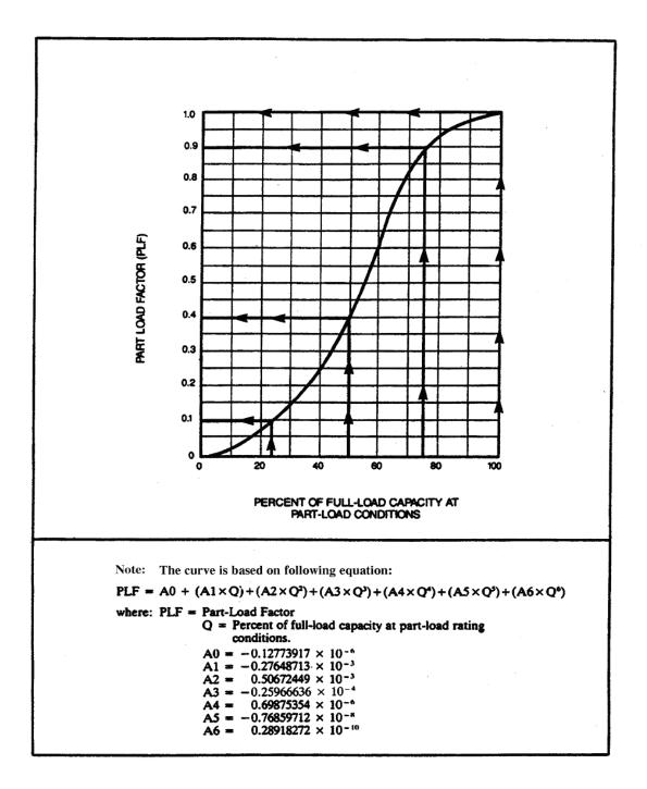
Figure C1. Part-Load Factor Example
