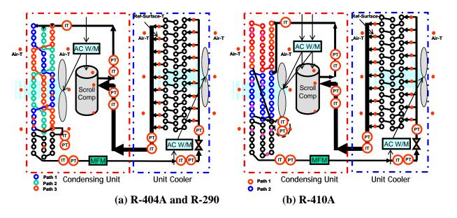
**Figure 9: Heat Exchanger Circuits and Instrumentation**
