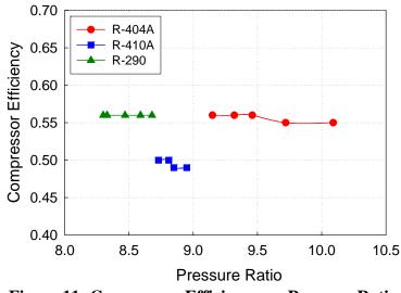
Figure 11: Compressor Efficiency vs. Pressure Ratio
