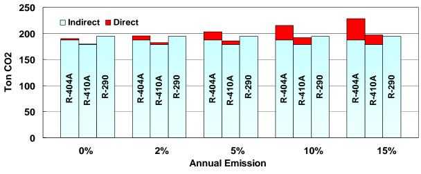
Figure 13: Comparison of LCCP at Various Annual Emissions (Based on the equal compressor efficiency and first cost)
