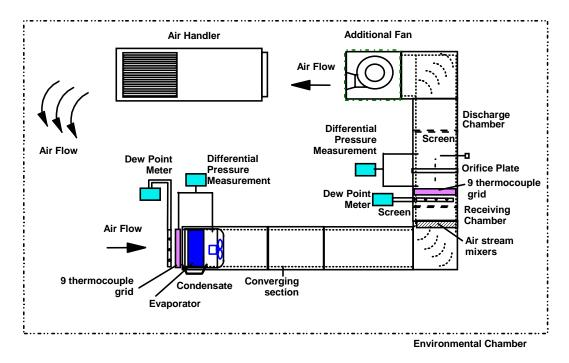
Figure 7: Test Facility for Unit Cooler
