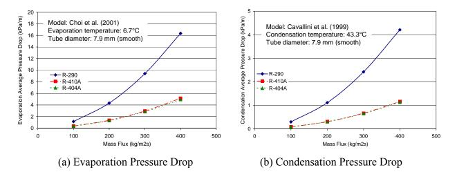
**Figure 5: Pressure Drop Characteristics of Refrigerants**
