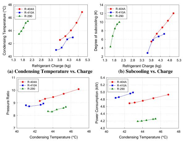
(c) Pressure Ratio vs. Condensing Temp. (d) Power Consumption vs. Condensing Temp.
