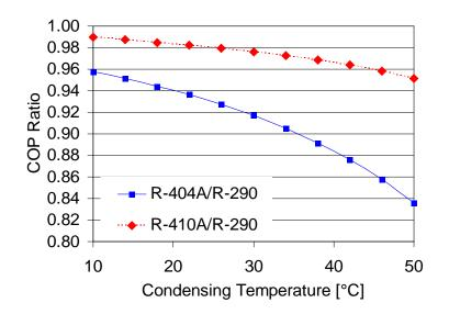
**Figure 3: Comparison of Theoretical Cycle Efficiency**
