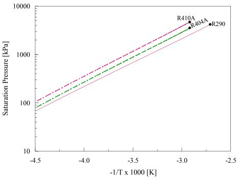
**Figure 1: Saturation Pressure of Refrigerants**
