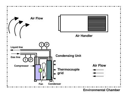
Figure 8: Test Facility for Condensing Unit
