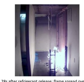
28s after refrigerant release; flame spread over the floor in the hallway towards the right wall.
