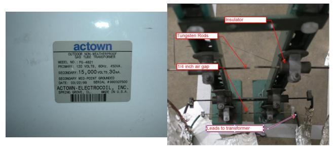
Figure 14 – Gas tube transformer and arc gap
