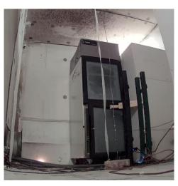
Flaring near pilot flame 5 seconds after the reach-in cooler door was opened.
