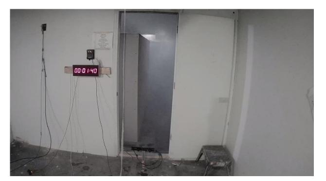
There was no ignition during this test. The candles at all locations flickered due to both wind and the presence of refrigerant. Candles at location A, B, and C remained lighted throughout the test. The candle at location D (shown here) was extinguished at 92 seconds after the start of discharge and 27 seconds before the end of the discharge.
