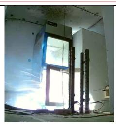
Flames 6s after reach-in cooler door; the flaming spread into the reach-in cooler.
