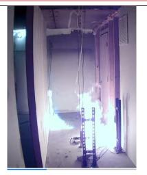
27s after refrigerant release; flame spread observed on the floor in the hallway toward the right wall.
