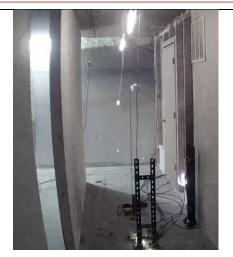
60s after refrigerant release; cheese cloth ignition all the way to the ceiling; all flaming ceased 76s after refrigerant release.
