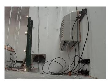
Floor camera view showing additional candles at location A and an additional electric arc at 24 inches. This frame is taken 2 seconds after the start of the discharge.
