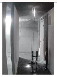
76s after refrigerant release; cheese cloth ignition all the way to the ceiling; all flaming ceased 84s after refrigerant release.
