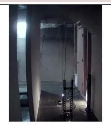
34s after refrigerant release flaming in hallway ceased; and flaming observed in the HVAC unit with smoke emitting from supply grill.
