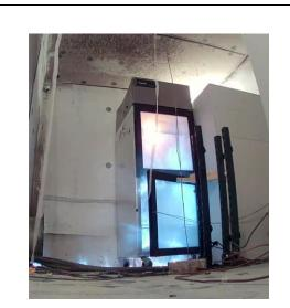
Flames 10s after reach-in cooler door is opened enter the cooler
