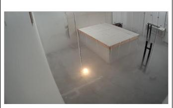
Ceiling camera view at ignition of candles and electric arcs 74 seconds after the start of discharge. Ignition time was delayed by 54 seconds to give time for the technician to leave the test room after closing the manual discharge valves.
