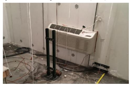
Figure 89 - Camera view of PTAC mounted in the center of the wall
