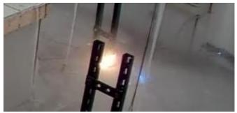
A small refrigerant flame was observed near location A. The cheesecloth was not ignited. The total flaming time for the refrigerant flame was 3 seconds.
