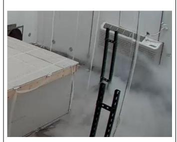
Ceiling camera view at 3 seconds after the start of the discharge. The jet moving to the right was due to the discharge impinging on a vertical support of the grill face.
