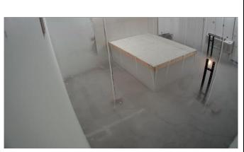
Ceiling camera view at ignition of candles and electric arcs 57 seconds after the start of discharge.
