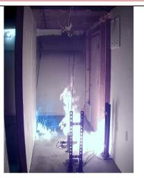
29s after refrigerant release; flame spread observed on the floor in the hallway twoard the right wall.
