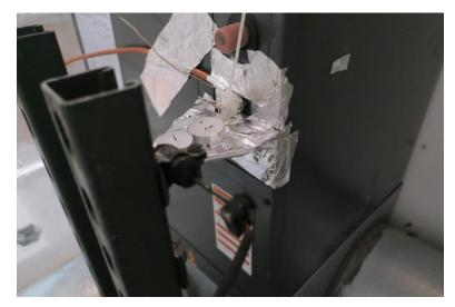
Refrigerant release location for leakage in A-Coil Scenario
