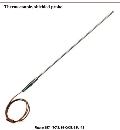
Ungrounded 1/8 inch diameter type K thermocouples were used to measure temperatures in the release and pressure tanks as well as the surrounding water baths.
