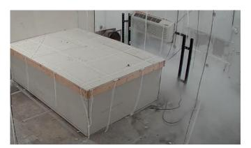
Ceiling camera view 10 seconds after the beginning of the discharge. While not apparent in a still frame, the video shows that the discharge location near the corner of the room is sweeping the mist away from that corner and entraining in fresh air from above the bed.
