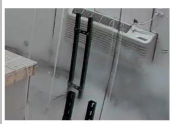
Ceiling camera view at 3 seconds after the start of the discharge. The jet moving to the right was due to the discharge impinging on a vertical support of the grill face.
