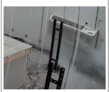
Ceiling camera view at 3 seconds after the start of the discharge. The jet moving to the right was due to the discharge impinging on a vertical support of the grill face.
