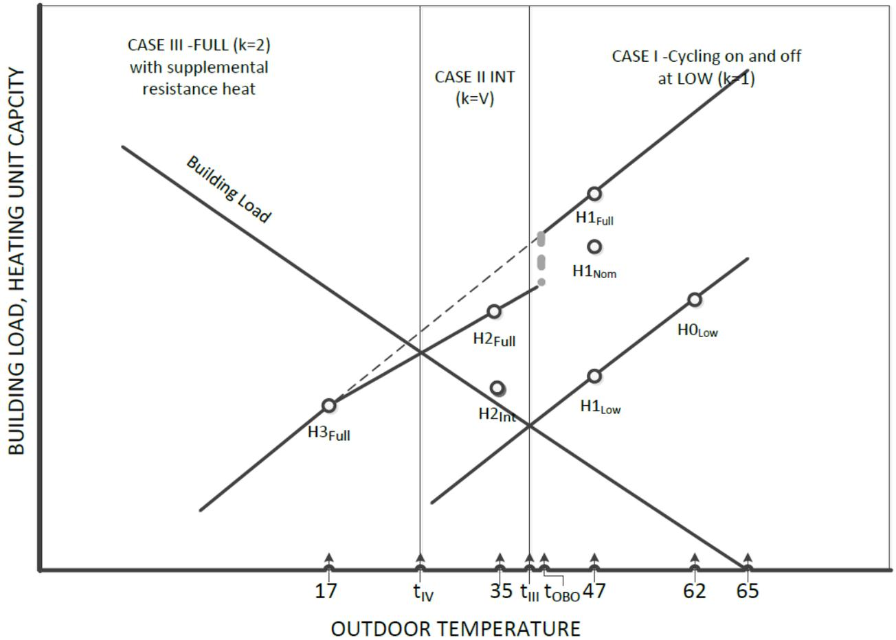
**Figure 9. Schematic of a Variable Speed Heat Pump Operation in Heating Mode**
