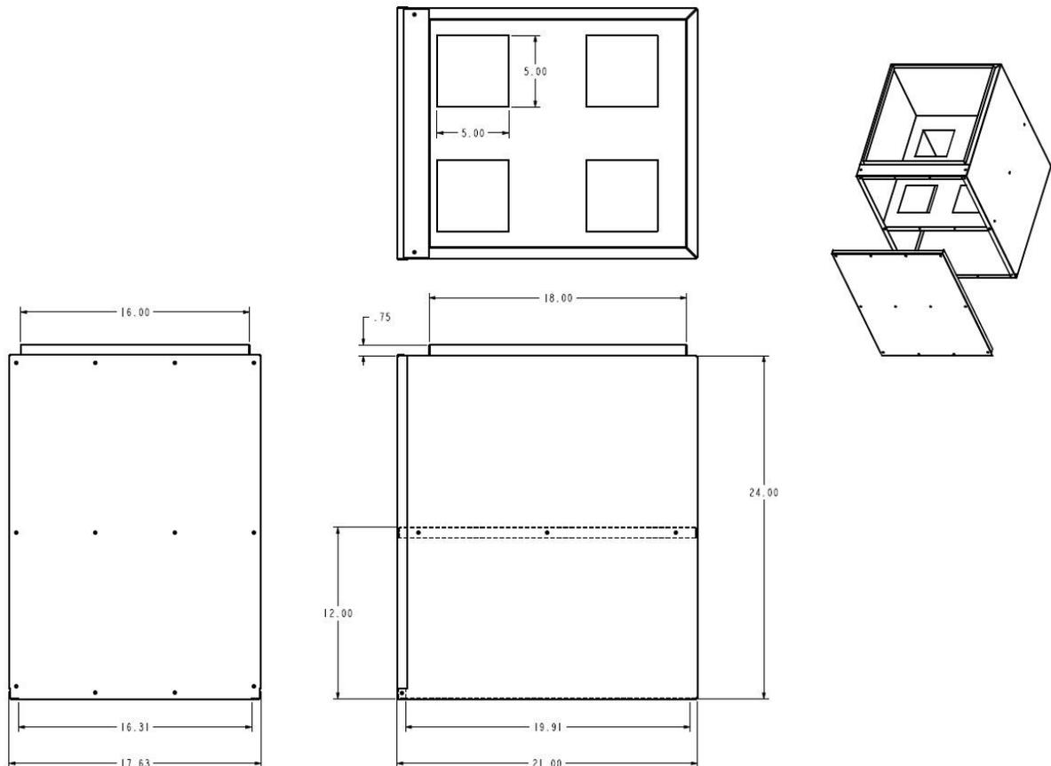
**Figure C1. Passive Pressure Drop Device**
