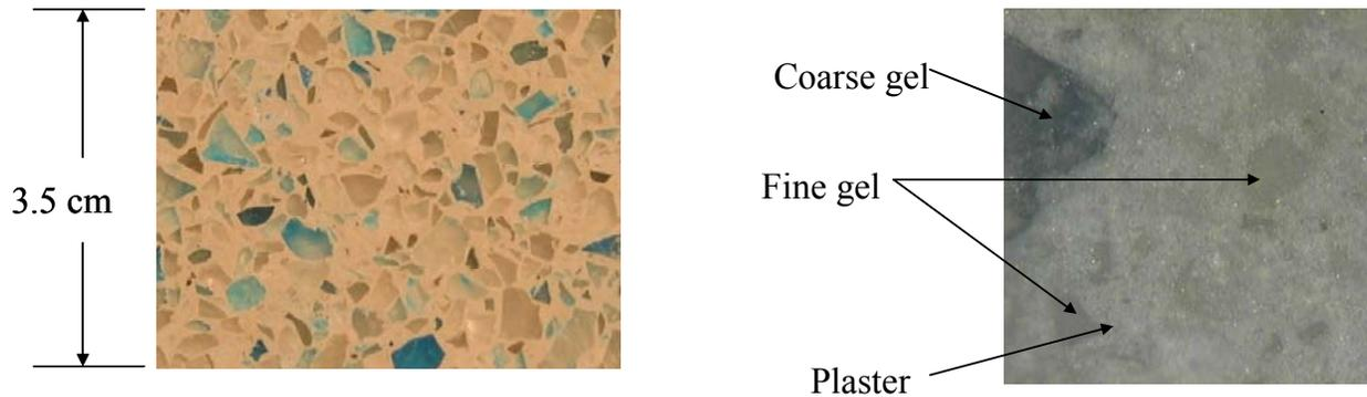
Figure 11: Left: Photo of sanded surface with coarse silica gel Right: Micrograph of silica gel concrete
