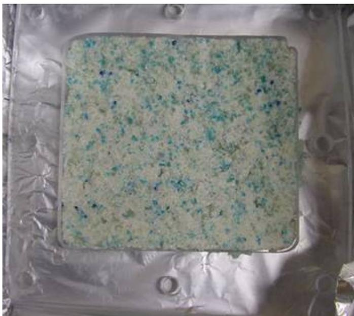
Figure C3: Agar- silica gel composite membrane
