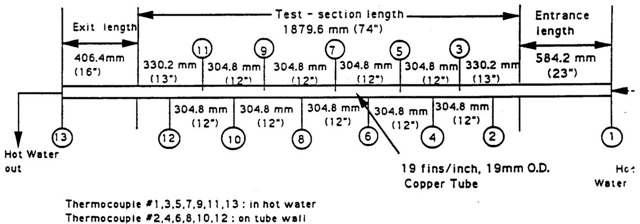
Fig. 2 Layout of thermocouples for the external boiling test section
