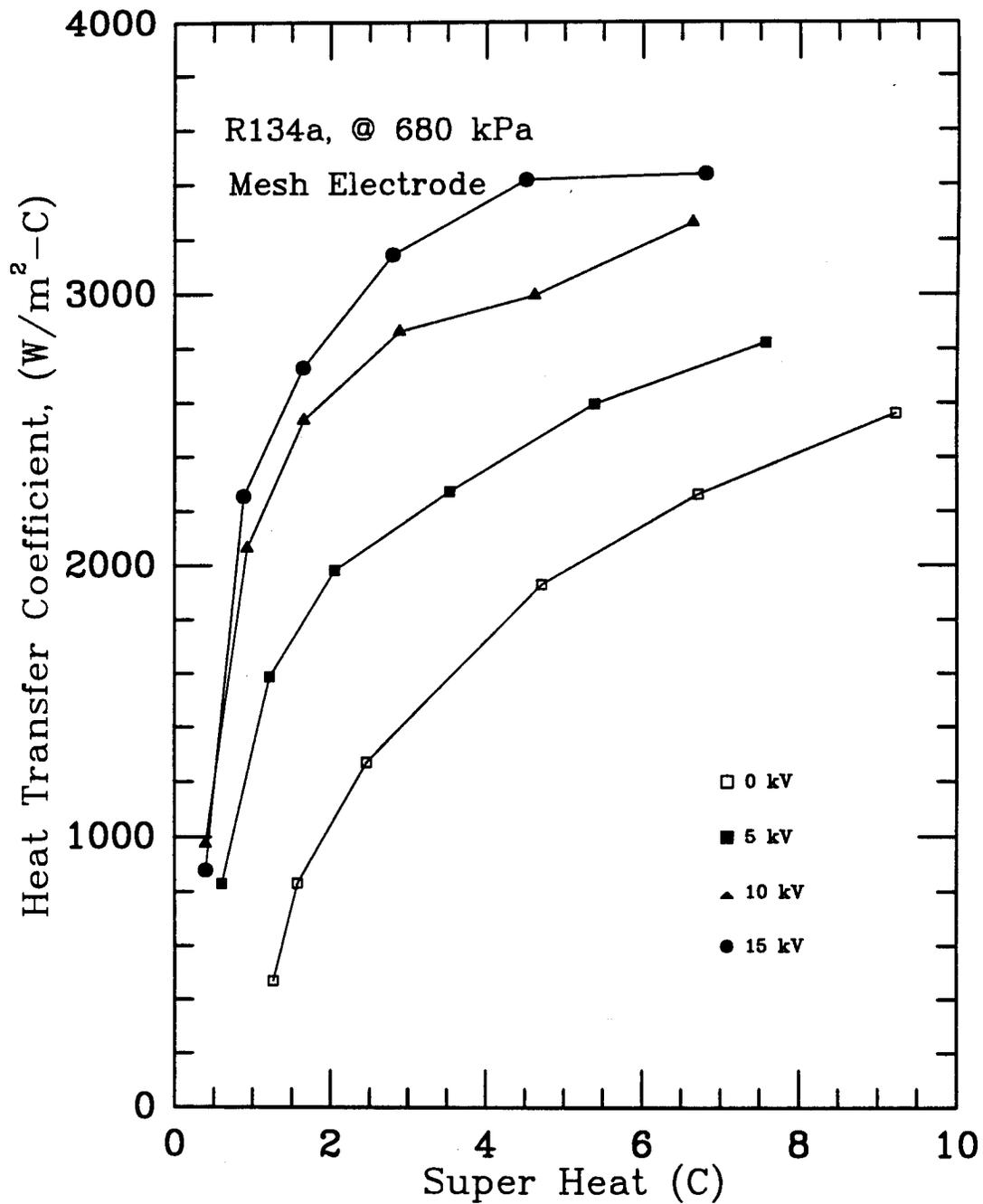
Fig. 7 EHD-enhanced external boiling of R-134a at P=680 kPa and  $T_{sat.}=25.85^{\circ}\text{C}$
