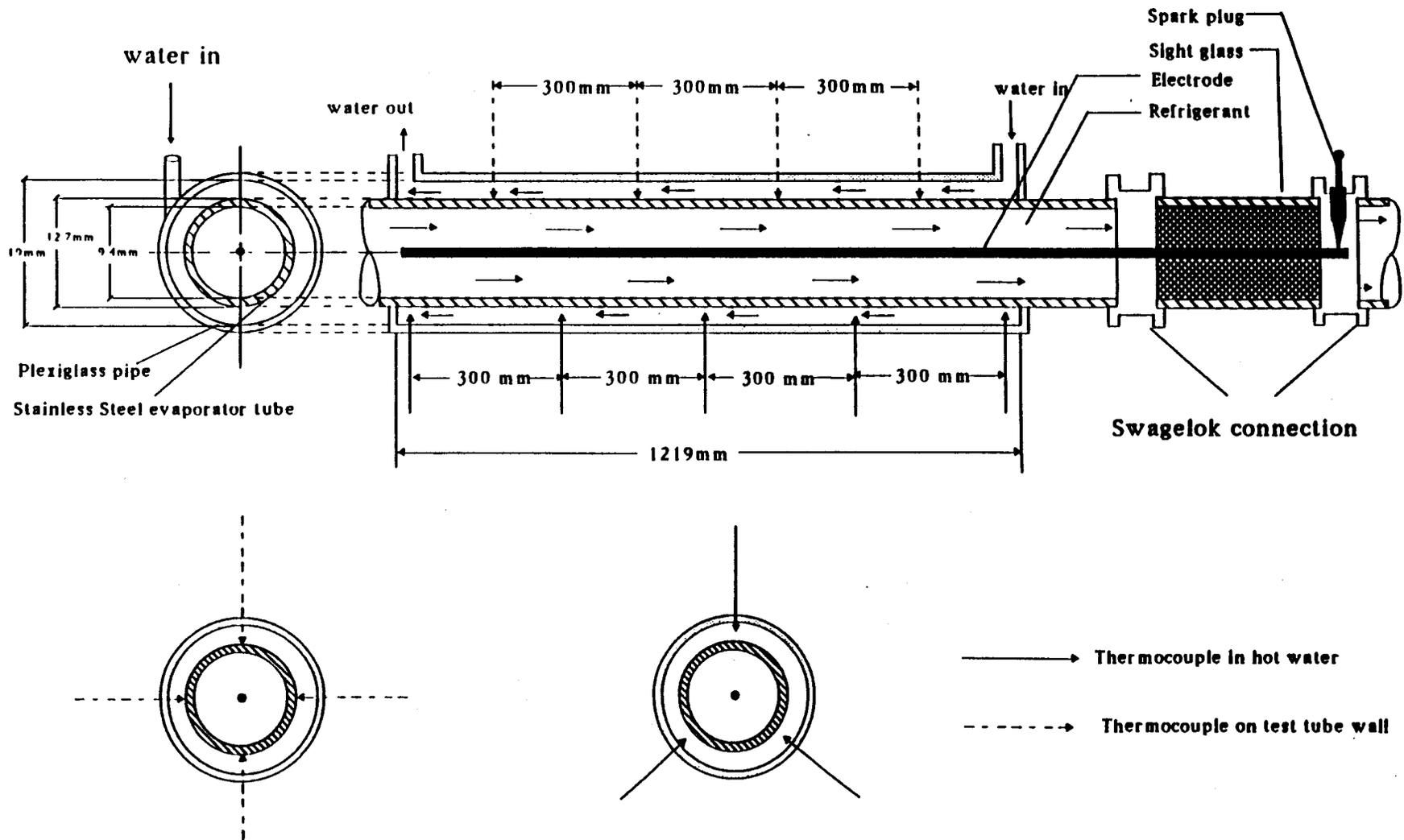
Fig. 10 Layout of test rig showing thermocouple locations
