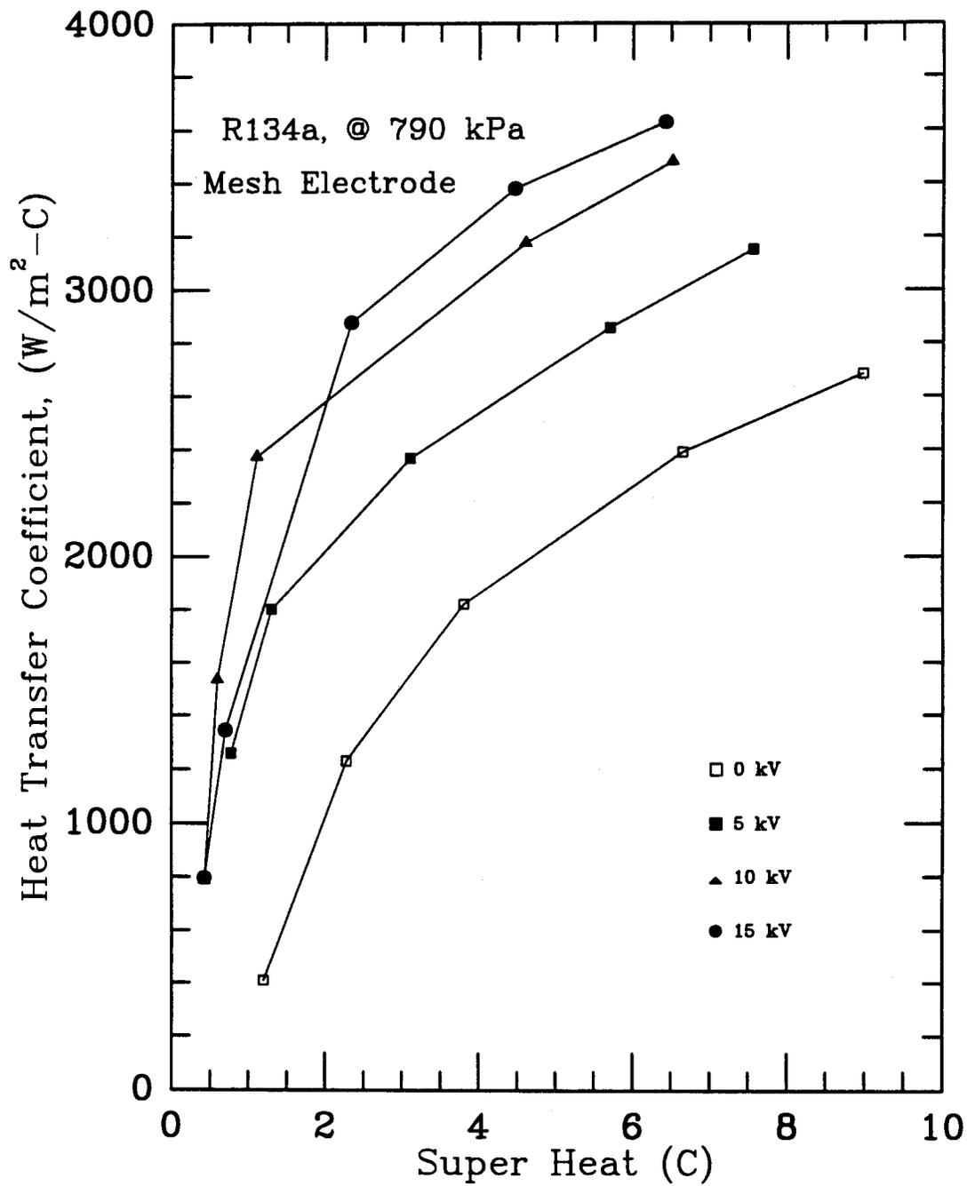
Fig. 8 EHD-enhanced external boiling of R-134a at P=790 kPa and T<sub>sat</sub>=30.85°C
