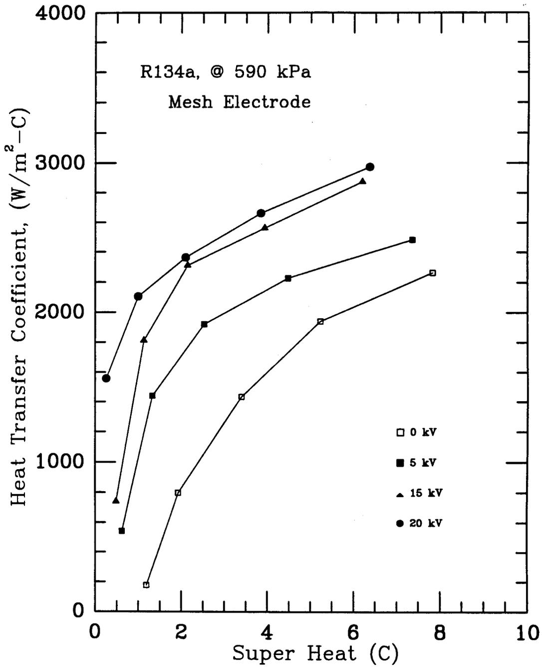
Fig. 6 EHD-enhanced external boiling of R-134a at P=590 kPa and  $T_{sat}=20.85^{\circ}\text{C}$
