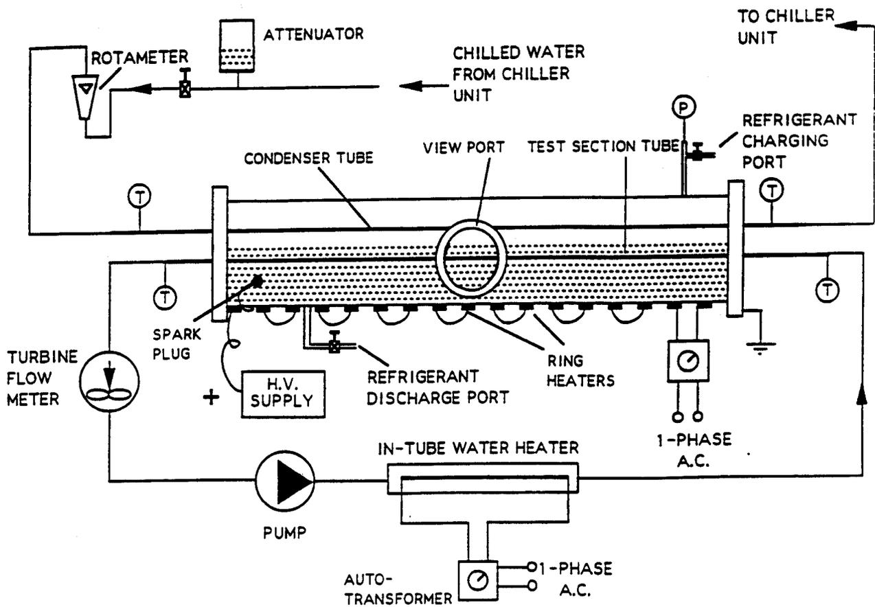
Fig. 1 Schematic of the external boiling test rig
