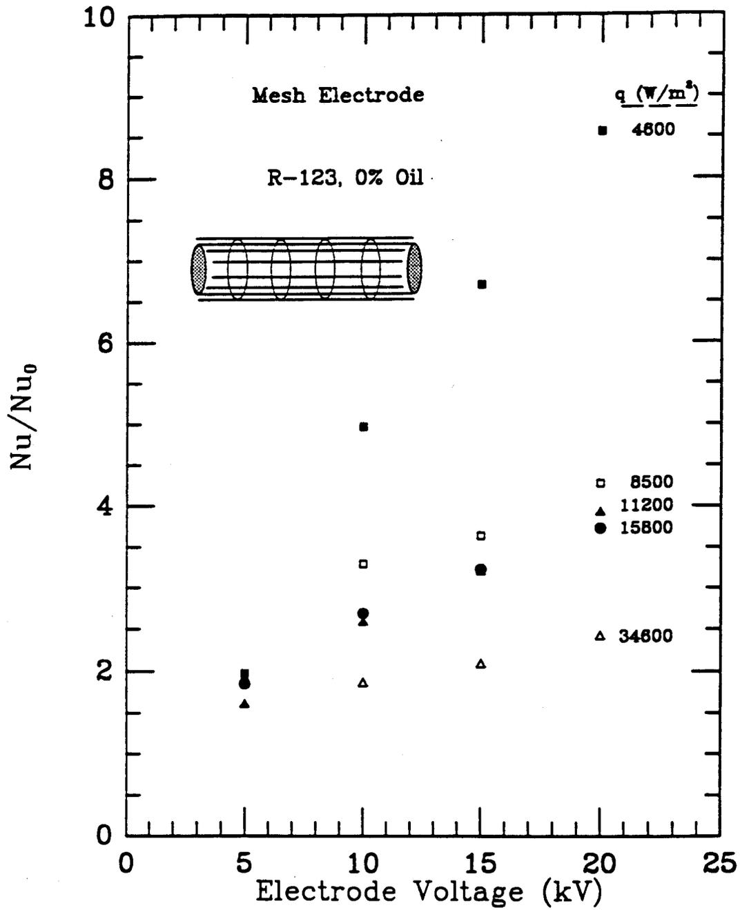
Fig. 4 EHD-enhanced external boiling of R-123 with wire mesh electrode at 0% oil
