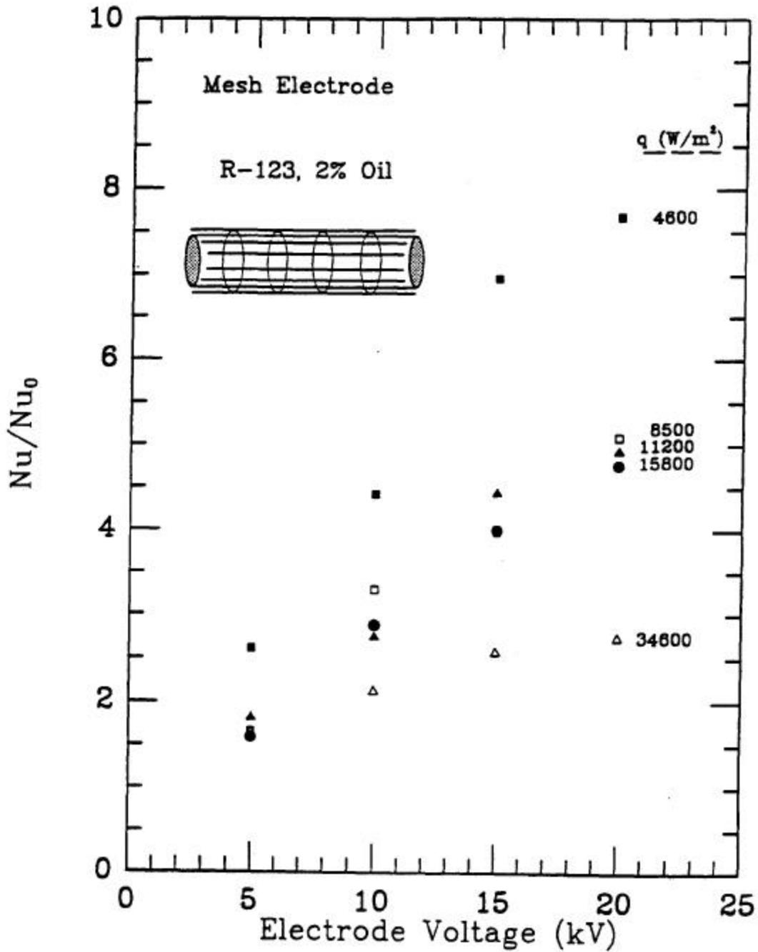
Fig. 5 EHD-enhanced external boiling of R-123 with wire mesh electrode at 2% oil
