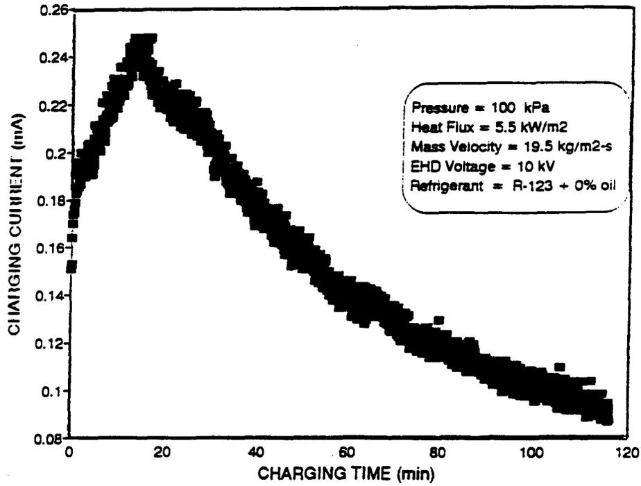
Fig. 12 Variation of EHD current for the in-tube boiling test section
