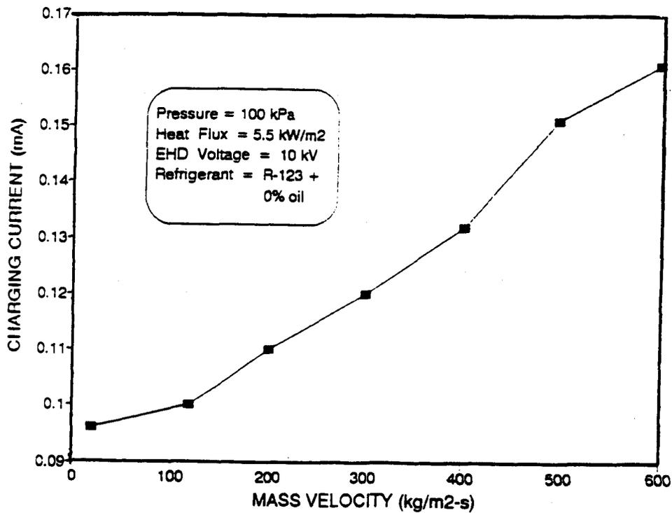
Fig. 13 Mass velocity vs. the EHD current for the in-tube boiling test section
