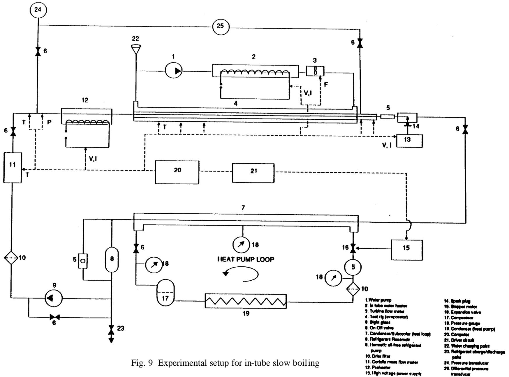
Fig. 9 Experimental setup for in-tube slow boiling
