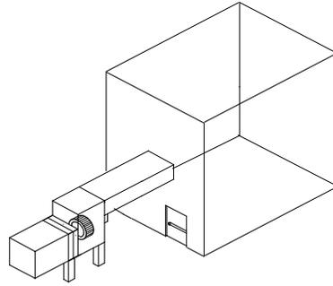
**Figure 3 – Concept Reverberation Room Ducted Discharge Test Set-up**
