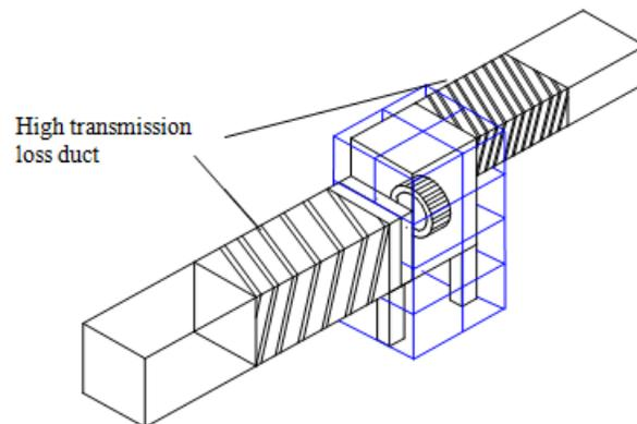
**Figure 8 – Concept Sound Intensity Casing Radiated Test Set-up**
