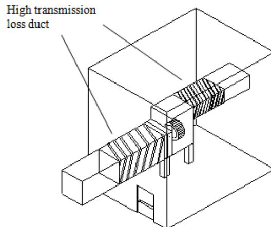
**Figure 7 – Concept Reverberation Room Casing Radiated Test Set-up**
