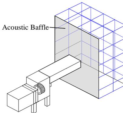
**Figure 4 – Concept Sound Intensity Ducted Discharge Test Set-up**
