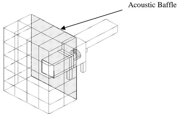
**Figure 6 – Concept Sound Intensity Ducted Inlet Test Set-up**
