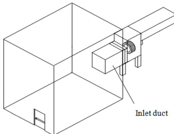
**Figure 5 – Concept Reverberation Room Ducted Inlet Test Set-up**
