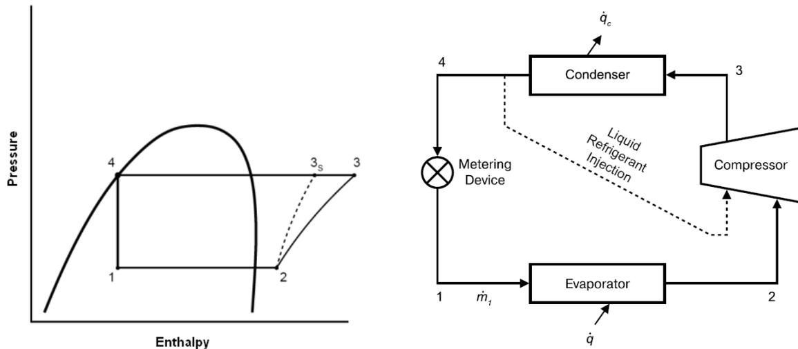
**Figure C5. Cycle Process for Subcritical Applications (AHRI Standard 571 Method 1)**
