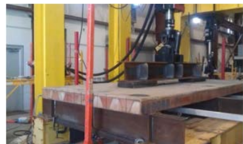
STRUCTURAL COMPOSITES PANEL UNDERGOING QUALIFICATION TEST AT FLORIDA DOT MOVEABLE DECK
