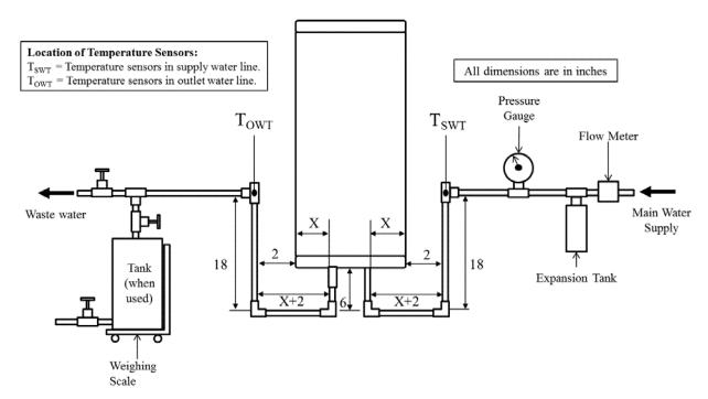
Figure 2.2. Set-up for thermal efficiency and standby loss test for water heaters equipped with vertical (bottom) connections
