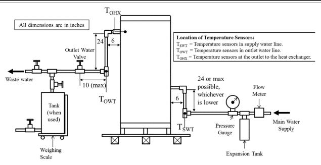
Figure 2.3. Set-up for standby loss test for electric instantaneous water heaters (other than storage-type instantaneous water heaters) equipped with horizontal connections not requiring a recirculating loop.
