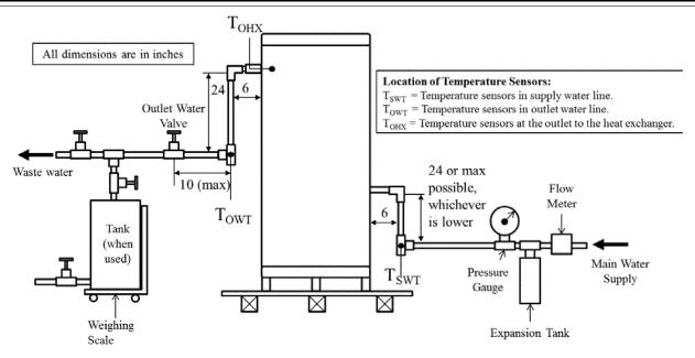
Figure 2.3. Set-up for thermal efficiency and standby loss test for gas-fired and oil-fired instantaneous water heaters and hot water supply boilers (other than storage-type instantaneous water heaters) equipped with horizontal connections not requiring a recirculating loop.
