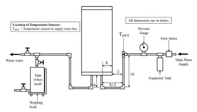
Figure 2.2. Set-up for standby loss test for electric storage water heaters equipped with vertical (bottom) connections
