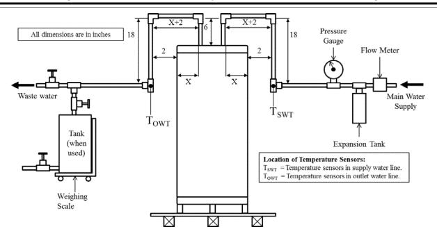
Figure III.1. Test set-up for gas-fired and oil-fired storage water heaters and storage-type instantaneous water heaters equipped with vertical (top) connections
