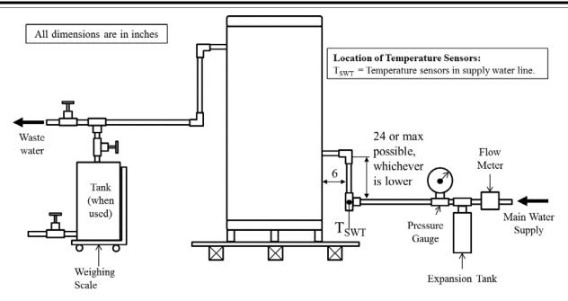
Figure 2.3. Set-up for standby loss test for electric storage water heaters equipped with horizontal connections
