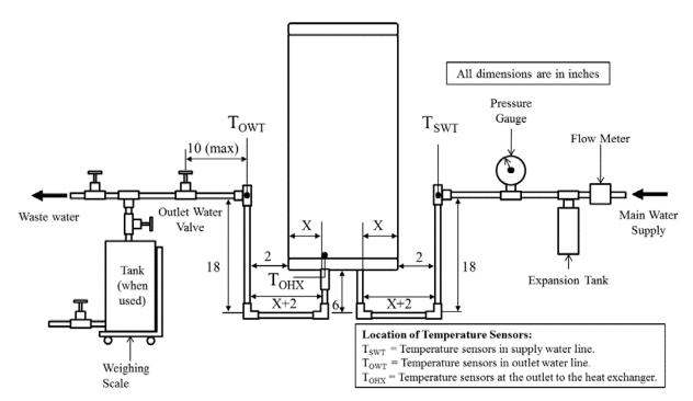
Figure 2.2. Set-up for standby loss test for electric instantaneous water heaters (other than storage-type instantaneous water heaters) equipped with vertical (bottom) connections not requiring a recirculating loop.
