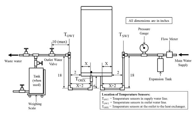
Figure 2.2. Set-up for thermal efficiency and standby loss test for gas-fired and oil-fired instantaneous water heaters and hot water supply boilers (other than storage-type instantaneous water heaters) equipped with vertical (bottom) connections not requiring a recirculating loop.
