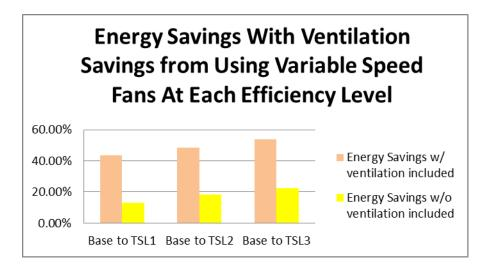
The assumptions made by the DOE on fan power depend on the design approach to increase IEER. There are many other ways to increase IEER other than through variable speed indoor fans, which is an effective approach, however, the timeline order with which the DOE includes them as an option on equipment may not be representative of how manufacturers design their units.
