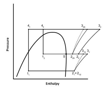
Figure C8. Cycle Process for Transcritical Application for Compressor Units with Manufacturer Specified or Supplied Subcoolers (AHRI Standard 571 Method 2)
