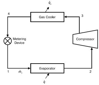
Figure C1. Single Stage Refrigeration Cycle Schematic with Thermodynamic State Point Numbers
