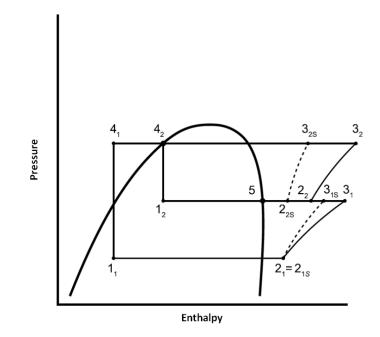
Figure C9. Cycle Process for Subcritical Application for Compressors Applied with Non-Specified Subcoolers (AHRI Standard 571 Method 3)
