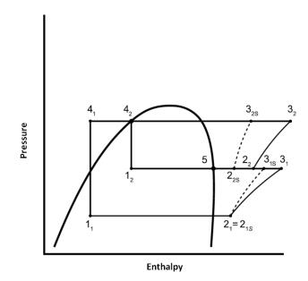
Figure C7. Cycle Process for Subcritical Application for Compressor Units with Manufacturer Specified or Supplied Subcoolers (AHRI Standard 571 Method 2)
