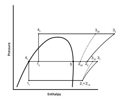
Figure C12. Cycle Process for Transcritical Applications for Compressors and Compressor Units Applied with Open Flash Style Liquid Subcoolers (AHRI Standard 571 Method 4)
