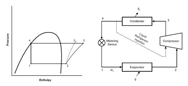
Figure C5. Cycle Process for Subcritical Applications (AHRI Standard 571 Method 1)
