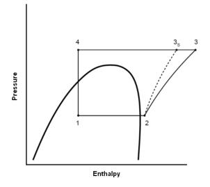
Figure C2. Single Stage Pressure Versus Enthalpy Diagram for the Refrigeration Cycle Shown in Figure C1
