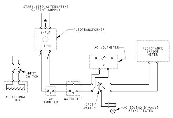
Figure C2. Typical Electrical Test Apparatus for an Alternating Current Solenoid Valve
