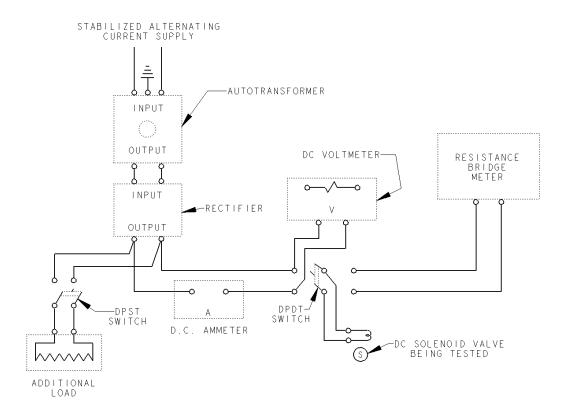
Figure C3. Typical Electrical Test Apparatus for a Direct Current Solenoid Valve
