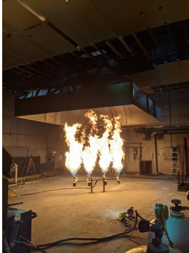
Figure 2 – ADD room Calorimeter hood with a calibration fire in progress
