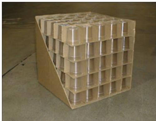
Figure 34 - Group A Plastic Commodity (partially cut box to show the cup arrangement)
