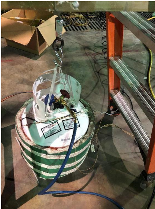
Tank Weighing and Heater Blanket
