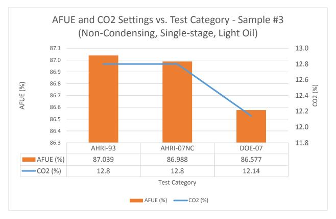
Figure 3 – AFUE and CO<sub>2</sub> Test Results for Sample #3 (Non-Condensing, Single-stage, Light Oil)
