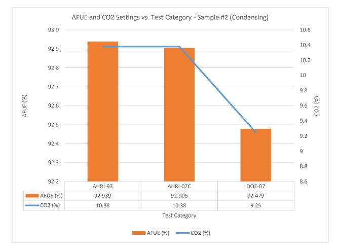
Figure 2 – AFUE and CO<sub>2</sub> Test Results for Sample #2 (Condensing, Step-Modulating, Natural Gas)
