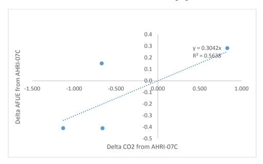
Figure 4 – Scatter Plot of Changes in AFUE and CO<sub>2</sub> from Testing, with Trendline
