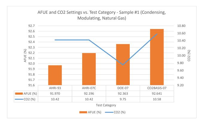
Figure 1 – AFUE and CO<sub>2</sub> Test Results for Sample #1 (Condensing, Step-Modulating, Natural Gas)
