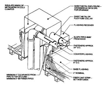
Clearances For Multiple Pipes -Between Pipes and From Walls And Curbs
