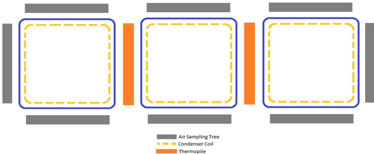
**Figure E4. Multiple Module Air Sampling Tree Placement Example**
