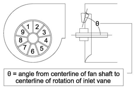
Figure 7. Dimensions for Inlet Vane Proportionality
