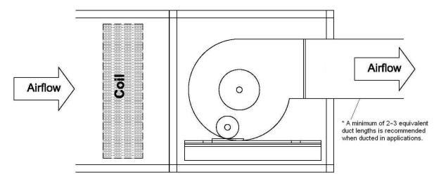
Figure 2. Ducted Fan Discharge - Horizontal Arrangement
