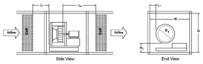
Figure C2. Dimensions Used for Proportionality Equations – Plenum Fan
