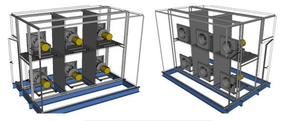
Figure C5. Example Contained Fan Array
