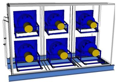
Figure C6. Example Uncontained Fan Array
