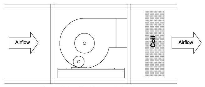
Figure 1. Unducted Fan Discharge - Horizontal Arrangement
