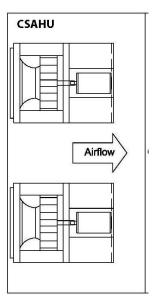
Figure 4. Single Outlet Test Unit Configuration for Single or Multiple Parallel Plenum Fans in CSAHUs with Full Face Opening Axial Discharge
