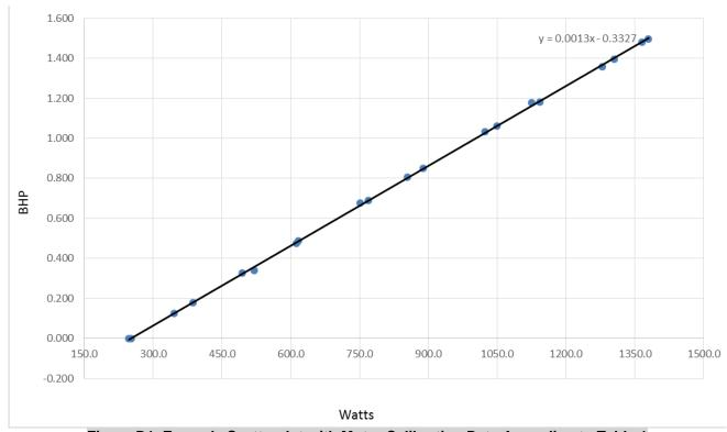
Figure D1. Example Scatterplot with Motor Calibration Data According to Table 1
