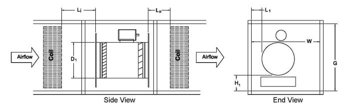
Figure C3. Dimensions Used for Proportionality Equations – Axial Fan
