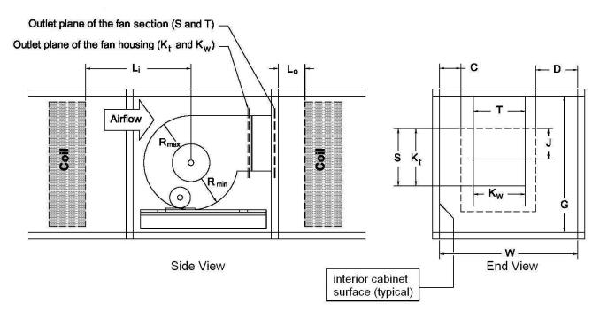
S and T are inside dimensions of the cabinet outlet. R  $_{min}$  and R  $_{max}$  are measured from the center of the shaft.
