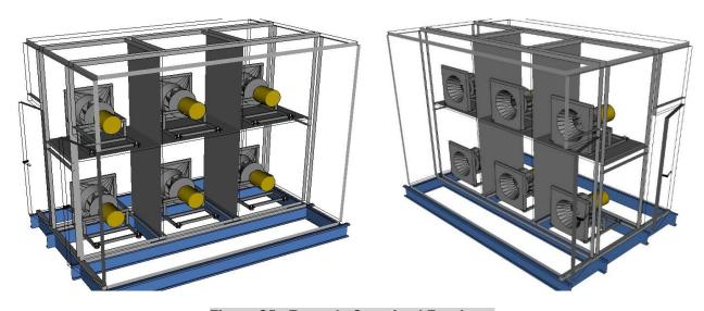
Figure C5. Example Contained Fan Array
