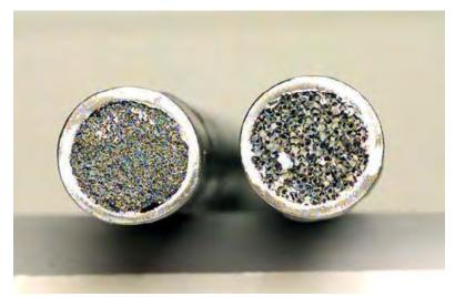
Figure 2.40 Metal-foam filled tubes using co-sintering technique. [107]
