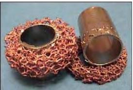
Figure 4.11 Copper foam brazed with Au/In brazed alloy (left) and after bond strength test (right) [205]
