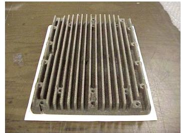
Figure 4.26 Metalized (plated) foam heat sink [132]
