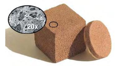
Figure 2.38 The structure of heat-pipe wicks (Metafoam<sup>®</sup>) [105]
