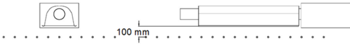
Figure 7 Measuring Plane of a Horizontally Mounted Low Intensity Infrared Heater
