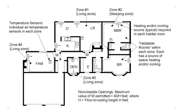
4. **Thermostats**. Each zone must be controlled by a central automatic dual setback thermostat that can control the conditioning equipment and maintain preset temperatures for varying time periods in each zone independent of the other. Thermostats controlling vented gas fireplace heaters that are not permanently mounted to a wall are acceptable as long as they have the dual setback capabilities.
